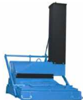
615 000 160 Towable Gallon Kettle Features a round tube factory tested heating unit that helps retain heat, one piece chimney cover, anti splash dual lids, front industrial jack leg and rear stabilizer leg. This kettle is ready to work with its burner hose and regulator, thermometer and 2-1/2" draincock.
