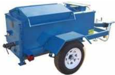
615 000 160 Towable Gallon Kettle Features a round tube factory tested heating unit that helps retain heat, one piece chimney cover, anti splash dual lids, front industrial jack leg and rear stabilizer leg. This kettle is ready to work with its burner hose and regulator, thermometer and 2-1/2" draincock.
